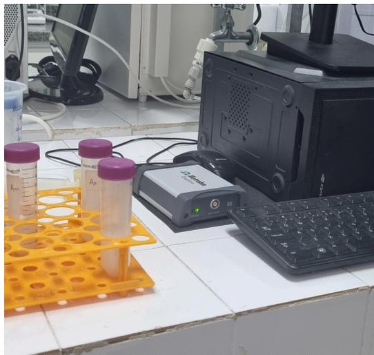
Fig. 2 - Potenciostato  $\mu$ Stat-i400s
